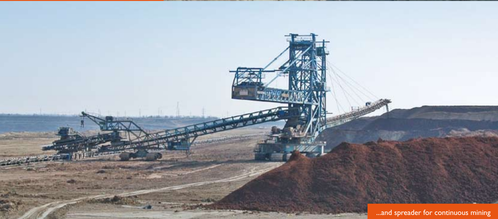
Bucket wheel excavator, belt wagon, conveyors...
