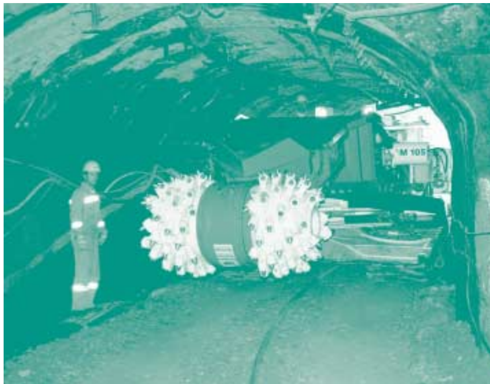
A selective cut heading machine in hard rock (Foto: Department of Mining Engineering)
