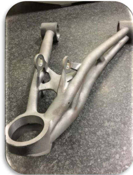
Figure 1: Demonstrator of the suspension arm showing the potential of AM production for automotive application
