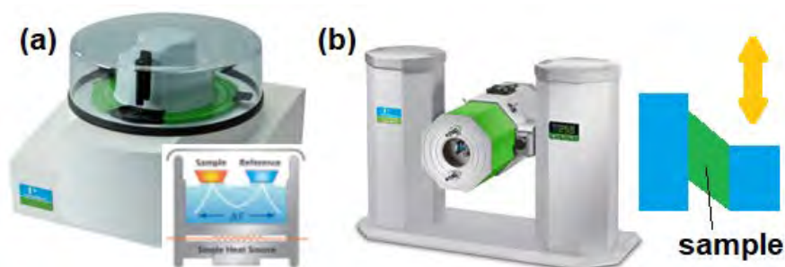
Fig. 1: measurement setup DSC (a) and DMA in shear mode (b)
