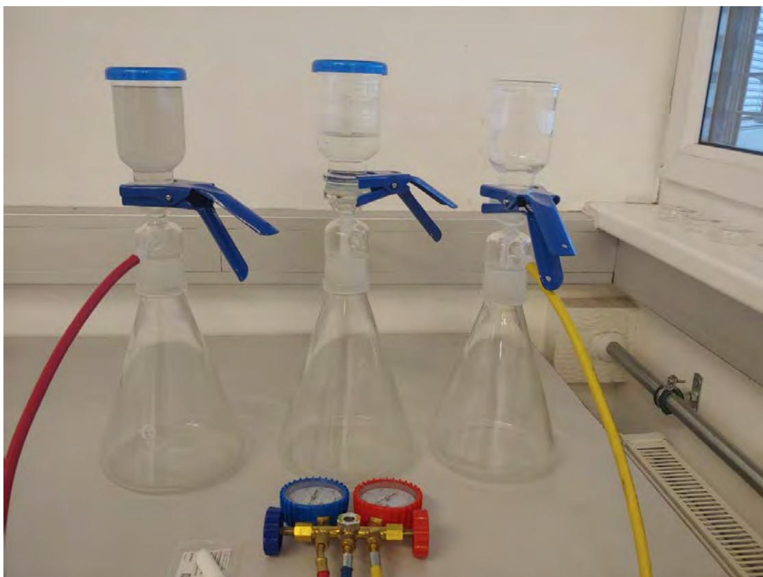
Fig. 1: Filtration setup using filters with decreasing pore size and vacuum pump assistance.
