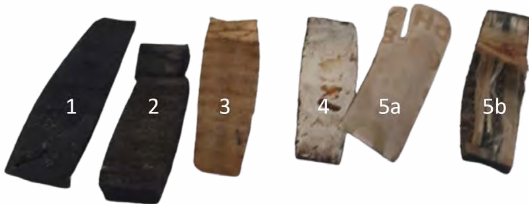
FFig. 2: Ski layers after chemical de-bonding, 1: Lining, 2: Wood Core, 3: Epoxy, 4: Aluminum, 5a+b: Cover layers
