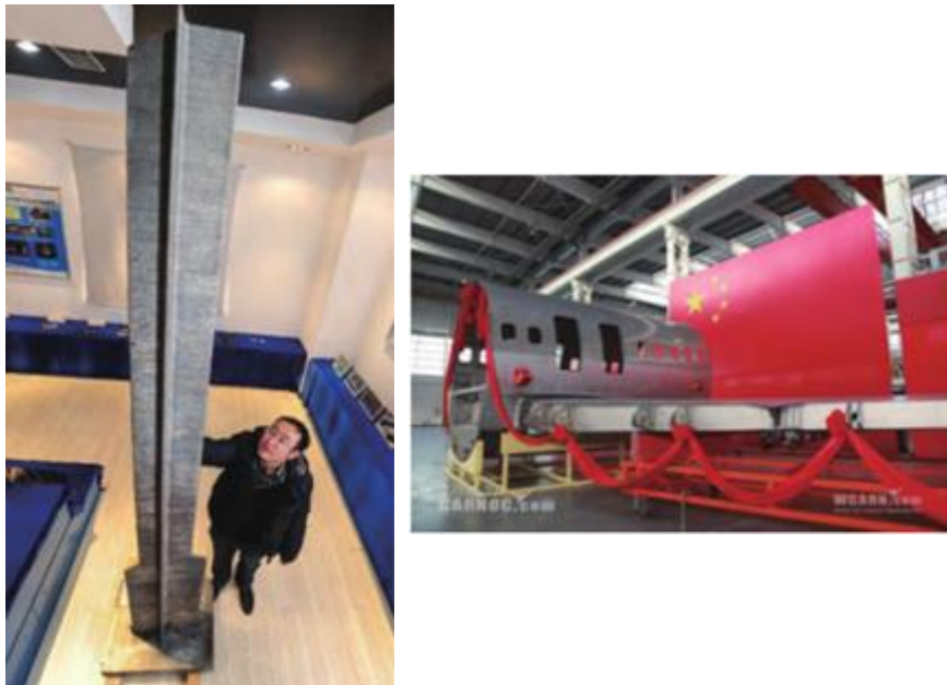
Fig. 1 The upper and lower margins of central wing of the the C919 large passenger aircraft manufactured by Northwestern Polytechnical University
