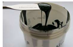
Paste made from oxide powder and ink vehicle
