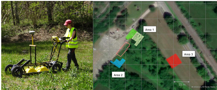
Above left: PulseEKKO geo-radar unit mounted on a non-ferrous cart with 500 MHz antennae and integrated Trimble RTK-GPS receiver. Right: Location map of three GPR survey areas conducted with the 500 MHz antennae near the Necropolis (red outlined area) at the Linea Cadorna, Ornavasso, Italy.
