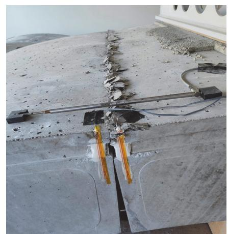
In addition to investigations aimed at determining the maximum loads that can be absorbed, special aspects such as the transfer of forces at the longitudinal segment joint are also considered.
